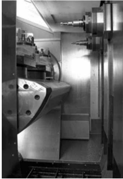
FIGURE 15.8 Interior of a twin spindle MQL machining center, showing horizontal spindle A-axis architecture, steep, unobstructed stainless steel walls, and an open bed over a chip conveyer. (From GROB, Grob Werke, Mindelheim, Germany.)
