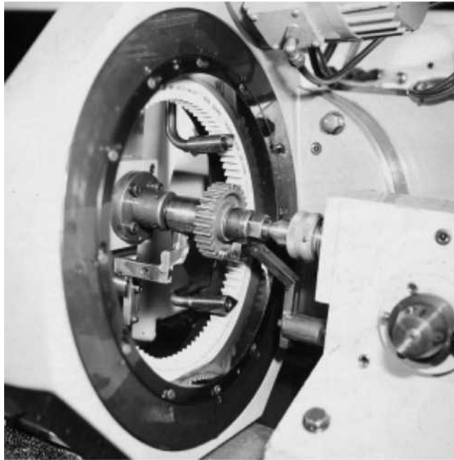
FIGURE 17.32 Honing an external gear using a honing ring. (From Sauter, Bachmann AG, Netstal, Switzerland.)
