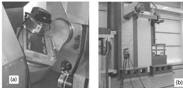
FIGURE 16.23 Illustration of the laser tracker: (a) on a rotary table of five-axis machine tool, (b) on a large machine tool. (Courtesy of Etalon AG, Braunschweig, Germany.)
