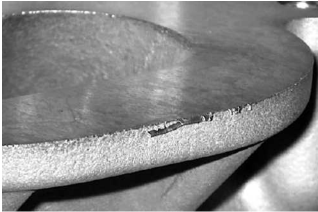
FIGURE 11.14 Rollover burr on a milled aluminum part.
