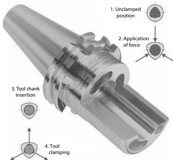
FIGURE 5.67 Precision polygonal mechanical actuated Tribos toolholder chuck. (Courtesy of Schunk Inc., Lauffen/Neckar, Germany.)
