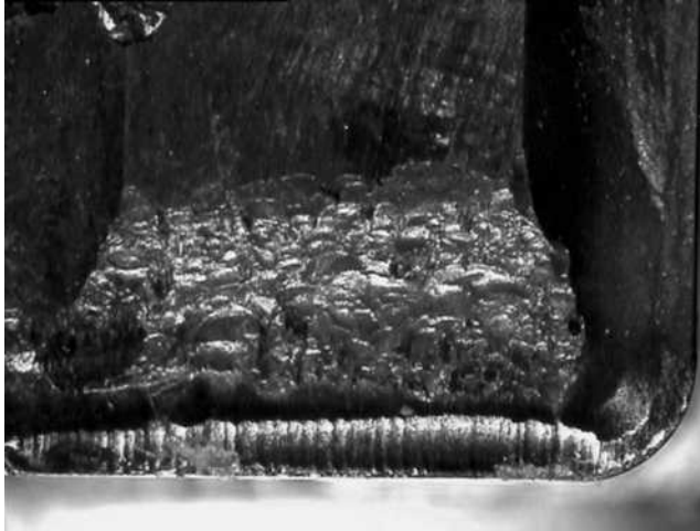
FIGURE 9.12 Chip hammering and cratering on a coated carbide insert used to machine a nickel alloy.
