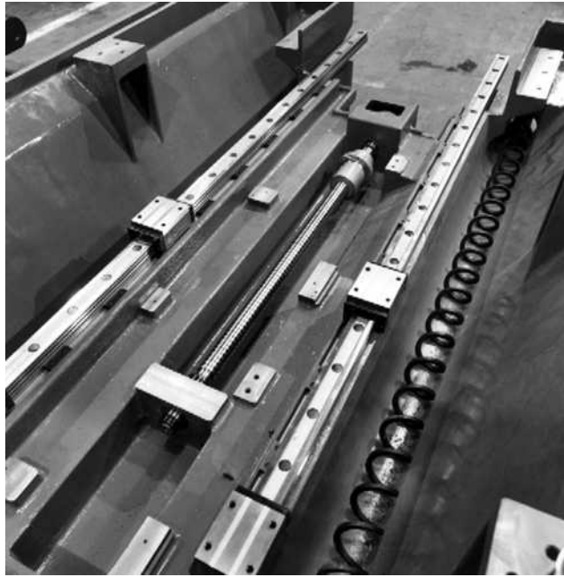
FIGURE 3.49 Typical arrangement of guideways, rolling bearing packs, and ball screw system in a machine bed. (Courtesy of Cincinnati Milacron, Cincinnati, OH.)
