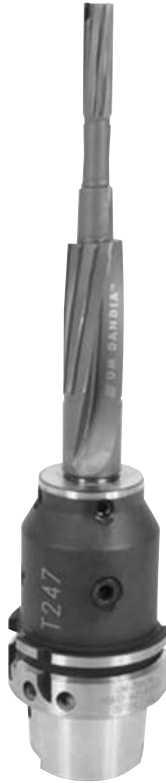
FIGURE 5.69 Steerable toolholder for transmission spool bore reamers and other rotating tools with critical runout requirements. Tightening the two rows of bolts in sequence while measuring runout with an indicator can be used to set up such tools with less than 5\text{ }\mu\text{m} TIR runout. (Courtesy of Kyocera Unimerco, Saline, MI.)
