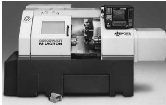
FIGURE 3.6 A CNC turning center with a main spindle and a subspindle for second-side capability, a rotating tooling turret, and a contouring C-axis. (Courtesy of Cincinnati Milacron, Cincinnati, OH.)
